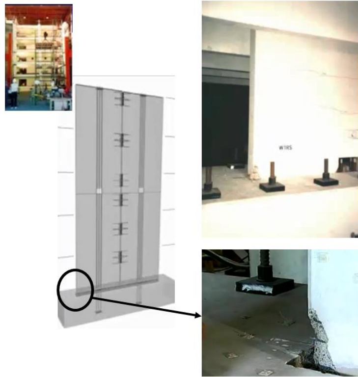
Figure 1-1. Post-testing observation on the rocking wall used in the 5-story Precast Concrete Building of the PRESSS Research program (Source: Precast Concrete Walls for Seismic-Resistant Design_from PRESSS Research to PreWEC webinar)
