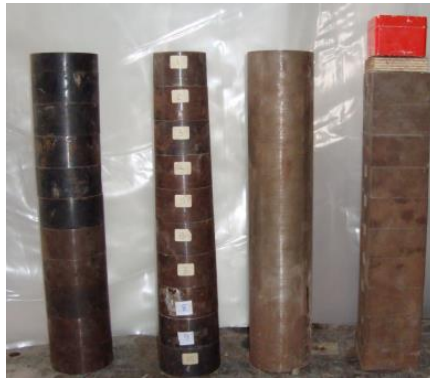
Figure 1-6. Specimens representing ancient free-standing monolithic columns subjected to ground motion during experimental and analytical studies conducted by Manos et al. (2013) in an effort to establish suitable numerical methods for estimating earthquake response of these simple ancient structural systems.
