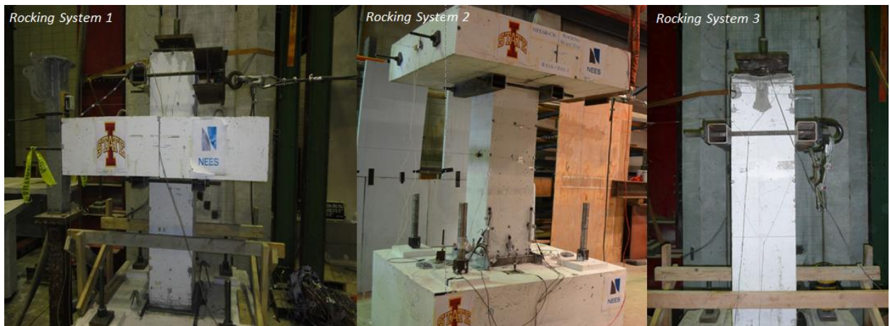
Figure 3-2. The three free rocking precast concrete units
